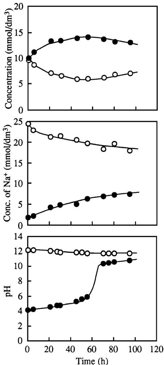
Figure 6 Changes in the concentrations of benzoic acid and Na<sup>+</sup> cation and pH values in the acidic (●) and alkaline (○) sides of PE-g-PDMA film with 5.5 mmol/g with time. (The initial pH value in the acidic side = 4.0 and the initial pH value in the alkaline side = 12.0.)
