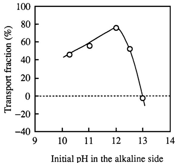
Figure 7 The effects of the initial pH value in the alkaline side on the transport fraction of benzoic acid. (The initial pH value in the acidic side = 3.2.)
