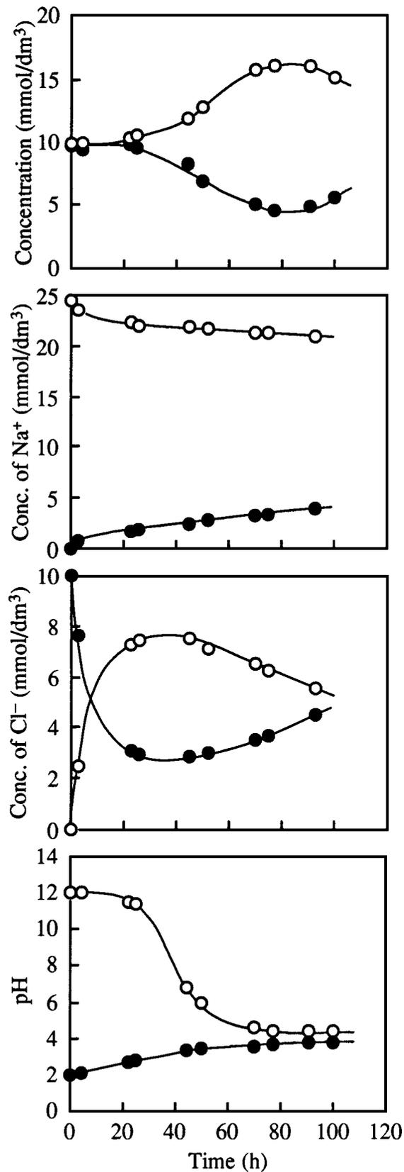
Figure 5 Changes in the concentrations of benzoic acid, Na<sup>+</sup> cation, and Cl<sup>-</sup> anion and pH values in the acidic (●) and alkaline (○) sides of PE-g-PDMA film with 5.5 mmol/g with time. (The initial pH value in the acidic side = 2.0 and the initial pH value in the alkaline side = 12.0.)
