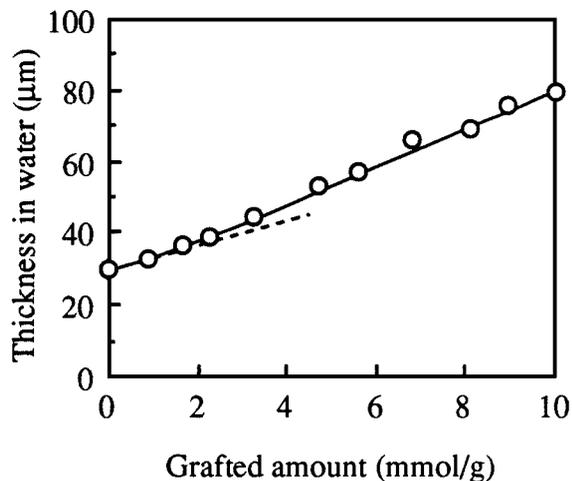
Figure 11 Change in the thickness with the grafted amount for PE-g-PDMA films swollen in water at 25 °C.
