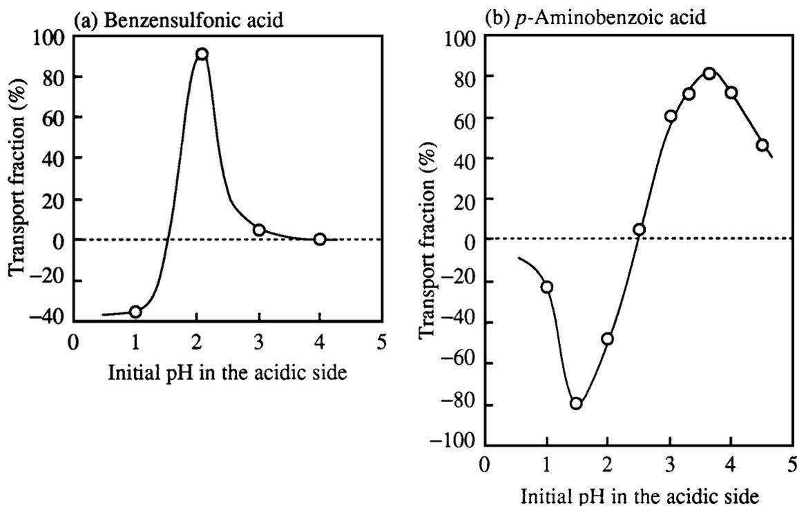
Figure 16 The effect of the initial pH value in the alkaline side on the transport fraction of (a) benzenesulfonic acid and (b) *p*-aminobenzoic acid. (The initial pH value in the alkaline side = 12.0.)
