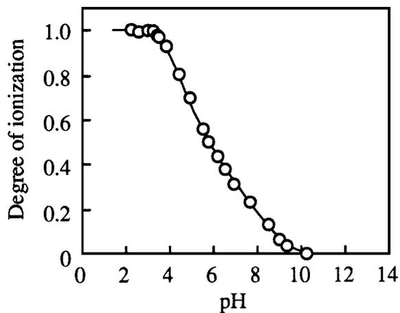
Figure 1 Change in the degree of protonation of dimethylamino group affixed to PDMA chains with pH value from colloid titration measurements with KPVS.
