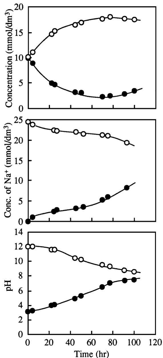
Figure 2 Changes in the concentrations of benzoic acid and Na<sup>+</sup> cation and pH values in the acidic (●) and alkaline (○) sides of PE-g-PDMA film with 5.5 mmol/g with time. (The initial pH value in the acidic side = 3.2 and the initial pH value in the alkaline side = 12.0.)
