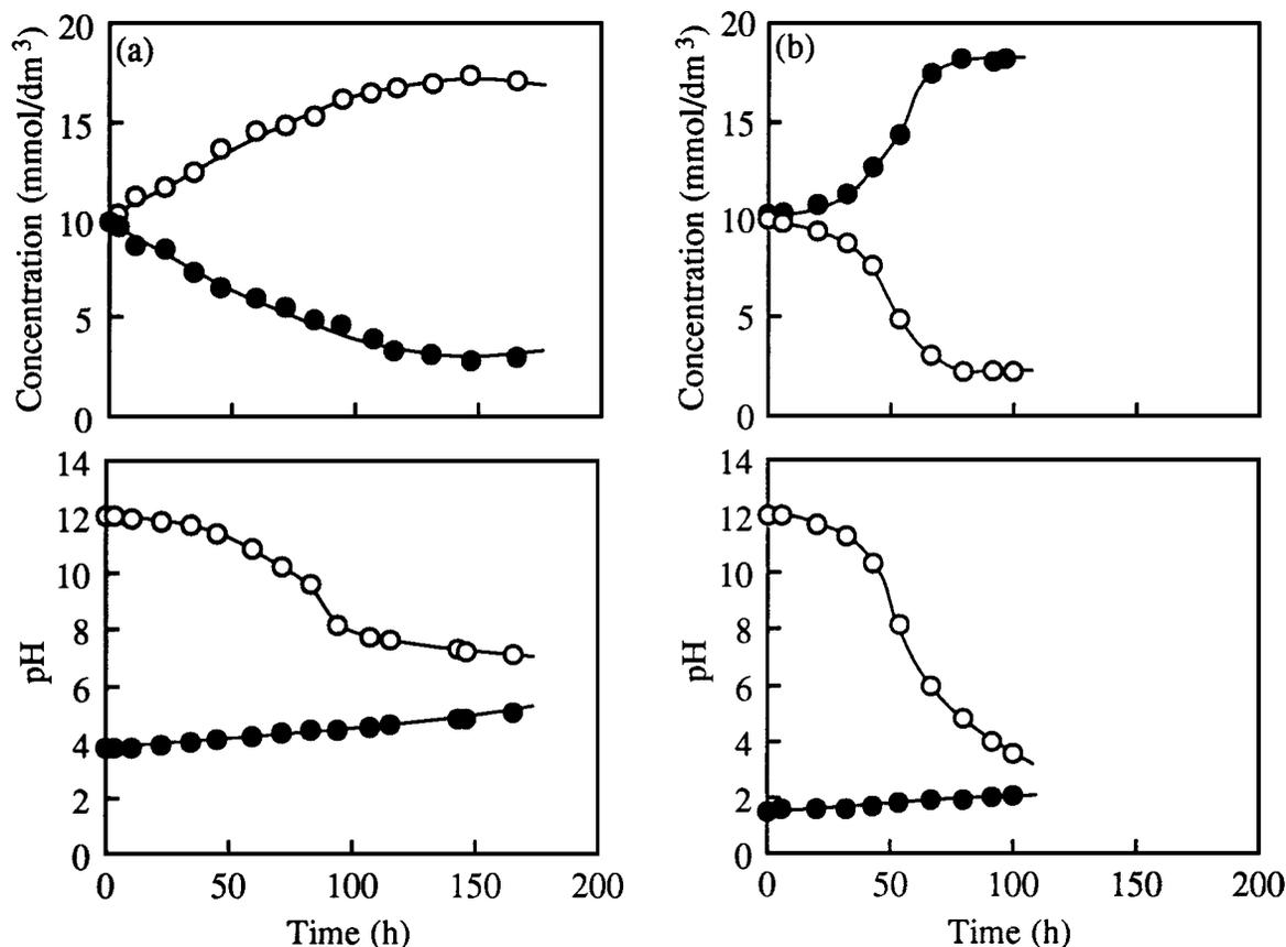
Figure 13 Changes in the concentration of *p*-aminobenzoic acid and pH values in the acidic (●) and alkaline (○) sides of PE-g-PDMA film with 5.5 mmol/g with time. (The initial pH value in the acidic side = (a) 3.8, (b) 1.5 and the initial pH value in the alkaline side = 12.0.)
