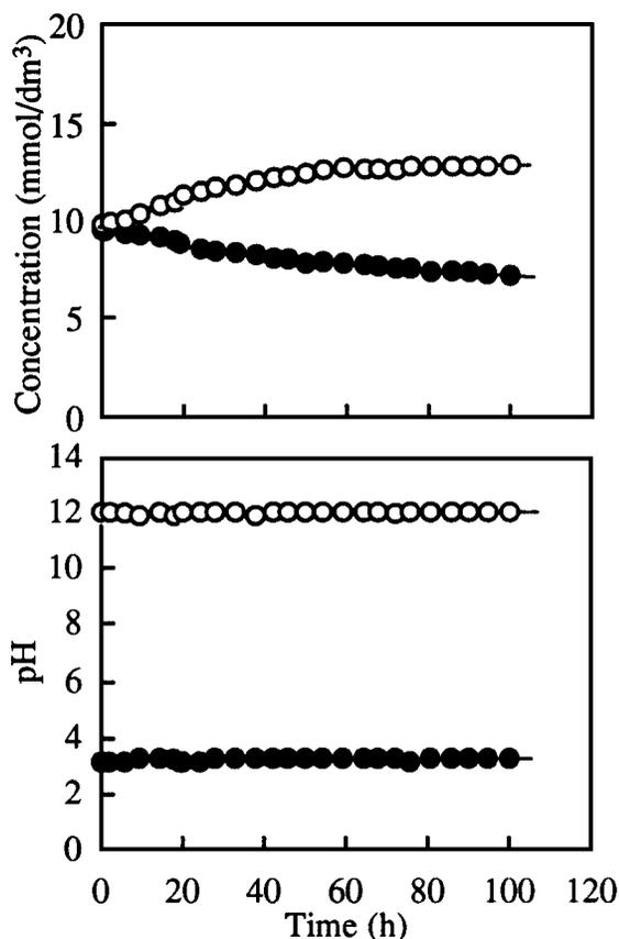
Figure 9 Changes in the concentration of benzoic acid and pH values in the acidic (●) and alkaline (○) sides of DMA-g-PE film with 5.5 mmol/g with time. (The initial pH value in the acidic side = 3.2, the initial pH value in the alkaline side = 12.0, and the initial pH values in the acidic and alkaline sides were kept constant by the addition of HCl and NaOH, respectively.)
