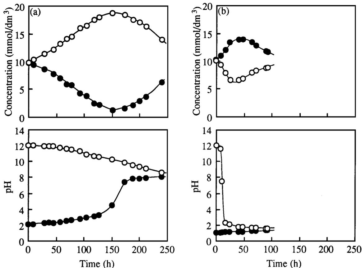
Figure 12 Changes in the concentration of benzenesulfonic acid and pH values in the acidic (●) and alkaline (○) sides of PE-g-PDMA film with 5.5 mmol/g with time. (The initial pH value in the acidic side = (a) 2.1, (b) 1.0 and the initial pH value in the alkaline side = 12.0.)
