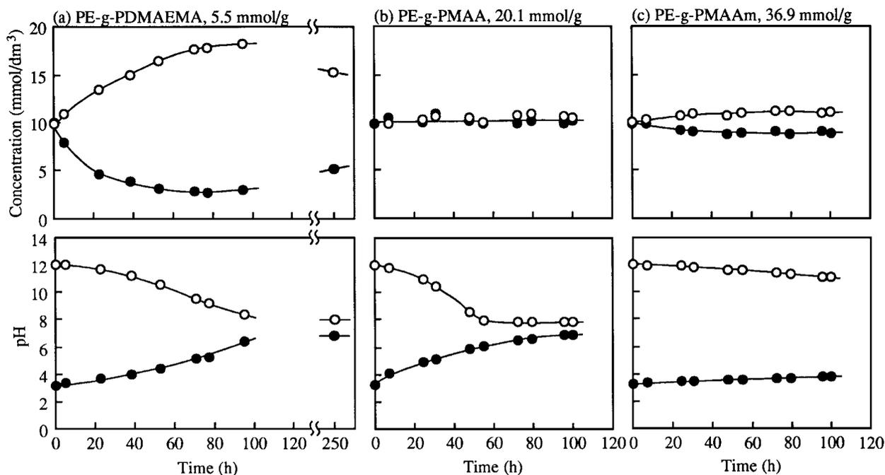
Figure 3 Changes in the concentration of benzoic acid and pH values in the acidic (●) and alkaline (○) sides with time for (a) PE-g-PDMA film with 5.5 mmol/g, (b) PE-g-PMAA film with 20.1 mmol/g, and PE-g-PMAAm film with 36.9 mmol/g.
