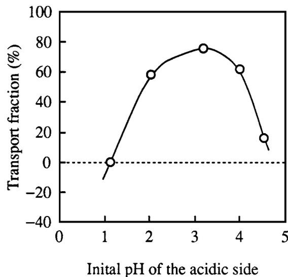
Figure 8 The effects of the initial pH value in the acidic side on the transport fraction of benzoic acid. (The initial pH value in the alkaline side = 12.0.)
