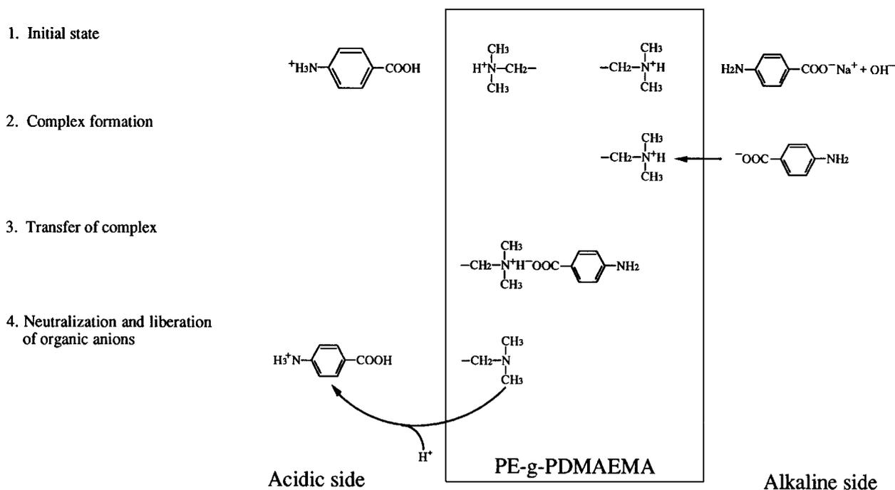
Figure 14 The mechanism of uphill transport of *p*-aminobenzoate anions through PE-g-PDMA film.
