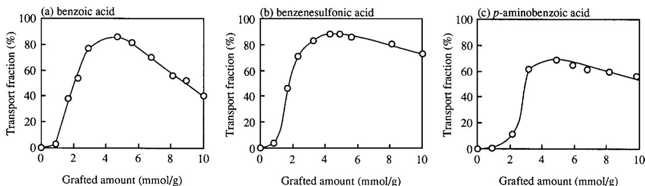
Figure 10 Changes in the transport fractions of (a) benzoic acid, (b) benzenesulfonic acid, (c) *p*-aminobenzoic acid with the grafted amount of PE-g-PDMA film.
