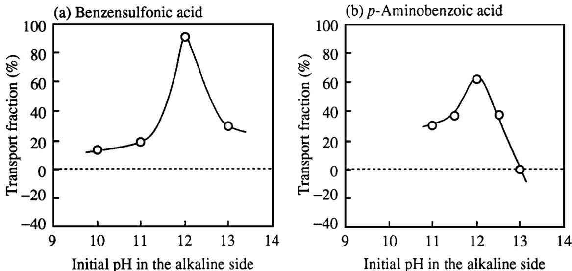
Figure 15 The effect of the initial pH value in the acidic side on the transport fraction of (a) benzenesulfonic acid and (b) *p*-aminobenzoic acid. (The initial pH value in the acidic side for benzenesulfonic acid = 2.1 and the initial pH value in the acidic side for *p*-aminobenzoic acid = 3.8.)
